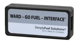
The Ward - Go Fuel - Interface (WGFI) is an integrated solution for odometer validation and OBDII data sharing between **Geotab** Go devices and Ward's Fuel Management system.
